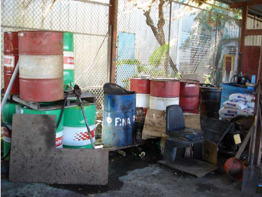
Picture 60. Used oil spill over the concrete floor at drum storage area.
