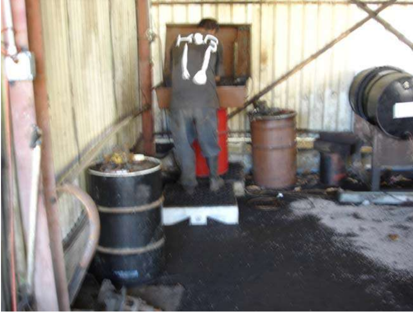
Picture 56. Absorbent material over stained soil at solvent wash station.
