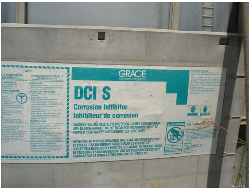
Picture 95. One of the chemicals used in connection with the concrete mixing plant.
